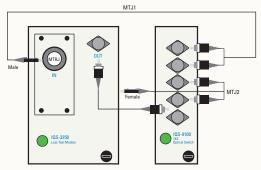
By doubling the number of switch ports, the system can be configured to accept both male and female multifiber connectors. The end result is faster and simpler testing in a single sequence.
